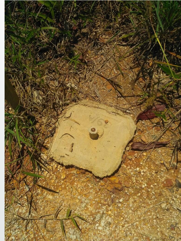
TBM ( Temporary Bench Marker)
